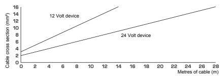
➤ Connect your cooling device as directly as possible to the battery terminal or to an outlet with a fuse of at least 15 A (12 V) or 7.5 A (24 V).
